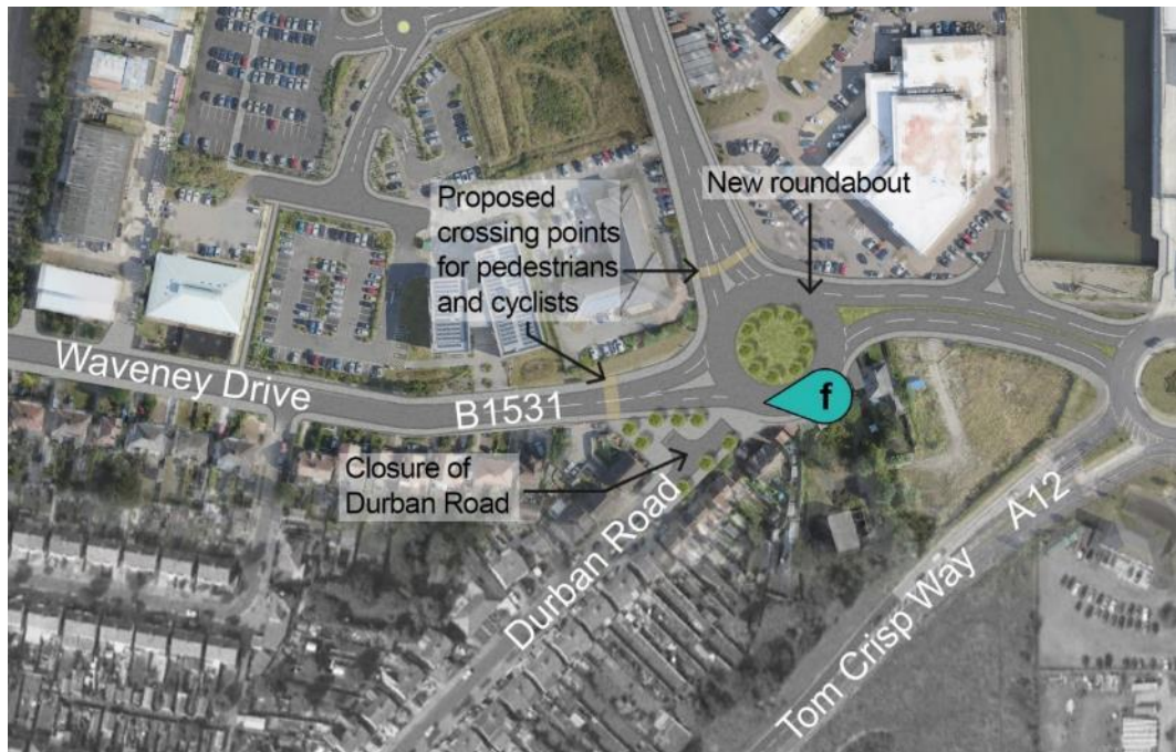
Figure 80: Southern approach area of the Scheme
